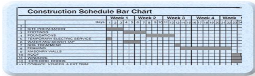
Figure 6. Typical Bar Chart for a Building Project
