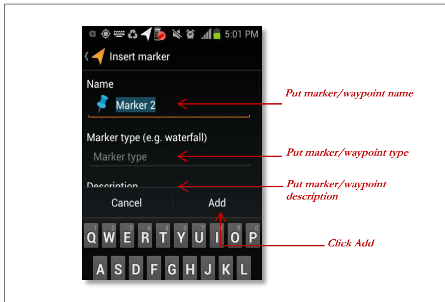
FIGURE 2.8 Input page of Marker/Waypoint Sample Geo-tagging Device: Samsung S2; Sample firmware version: ICS
